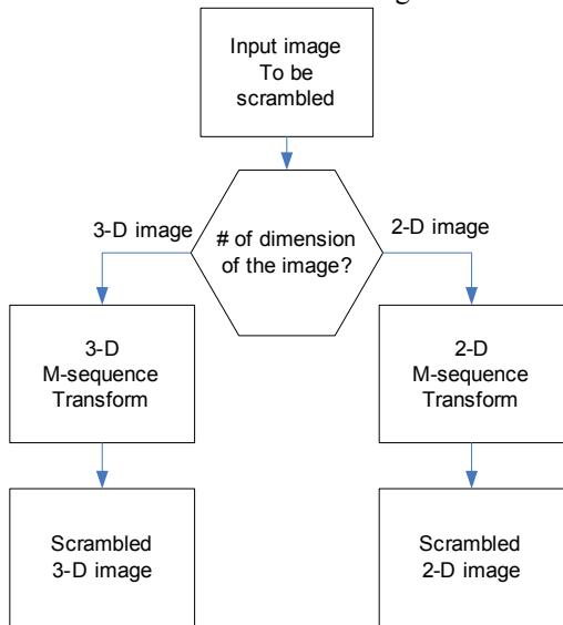
Figure 1. Block diagram of image scrambling algorithm
